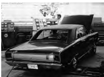
MR. NORM'S 1967 DART GSS 383 PROTOTYPE ON CLAYTON DYNAMOMETER GRAND SPAULDING DODGE
